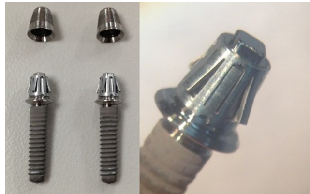
Figure 2. RODO devices show no signs of corrosion after 30 days of being fully immersed in 0.9% NaCl PBS solution.
